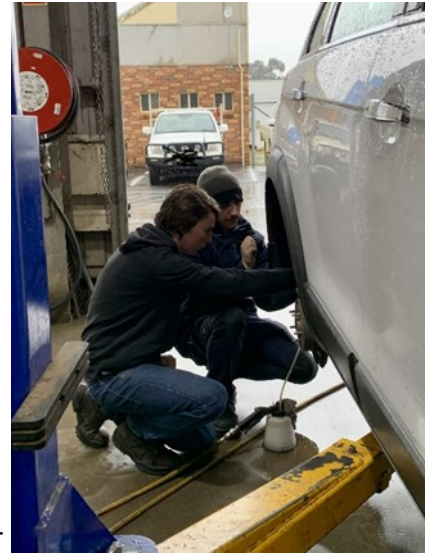
Tom being shown how to change brake fluid.
